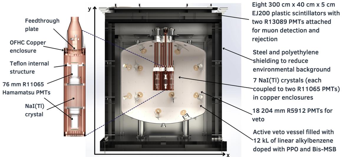
**Figure 2:** Cutaway render of the SABRE experiment annotated with the main components. Enlarged on the left is a cutaway of one of the seven target crystal modules.
