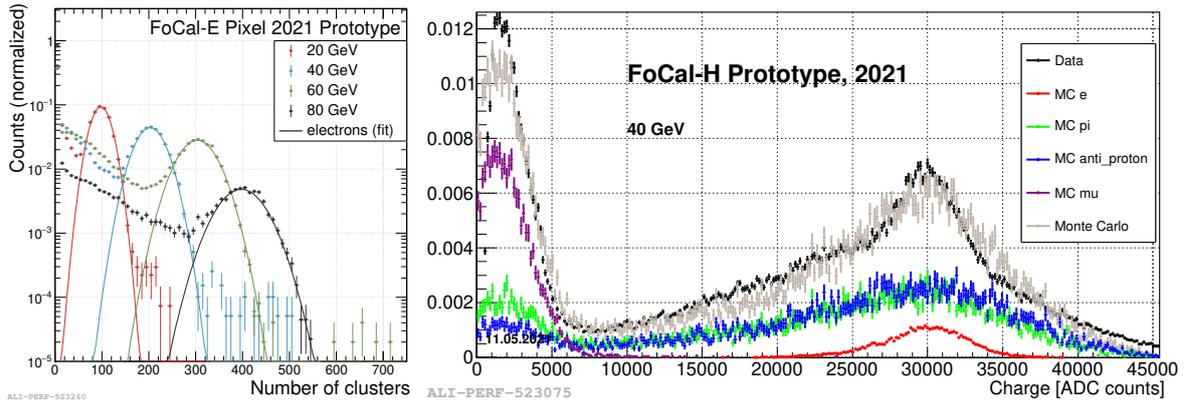
**Figure 3:** Left: Number of pixel clusters in FoCal-E Pixel layer 10 for energies of 20, 40, 60, and 80 GeV. The electromagnetic shower component is fitted with a gaussian function. Right: Measured signal in FoCal-H. A template fit with simulated signal of various particle types was applied to the dataset.
