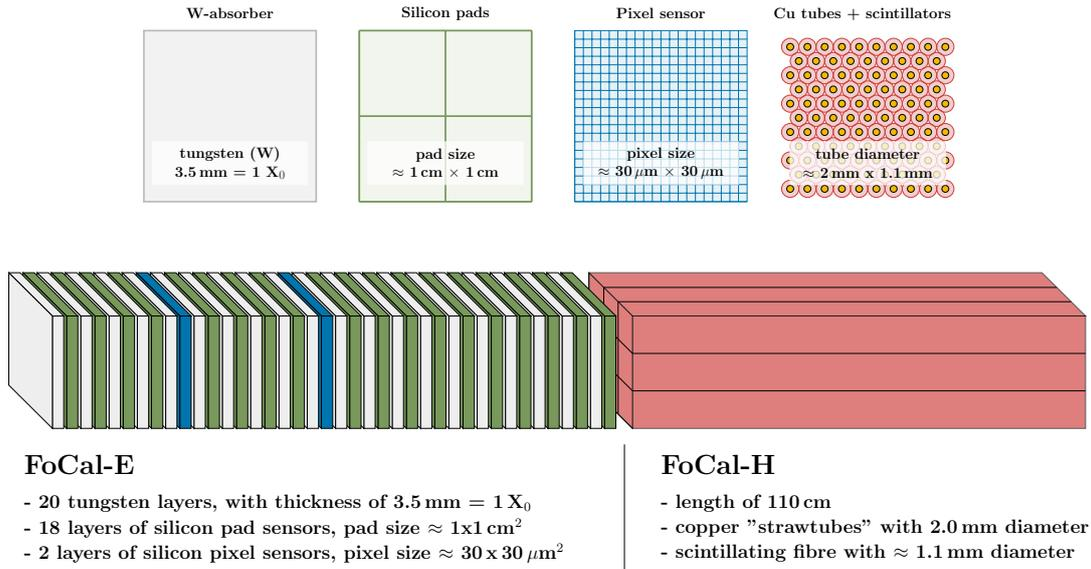
**Figure 1:** Detector design of the ALICE FoCal. A silicon-tungsten sampling electromagnetic calorimeter (FoCal-E) is followed by a scintillating-fibre-copper hadronic calorimeter (FoCal-H). Not to scale.
