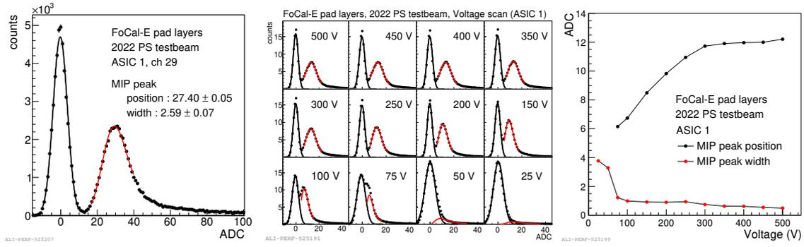
**Figure 4:** Left: MIP signal peak measured in ADC units. Center: Evolution of MIP signal peak for various sensor bias voltages between 0 and  $-500$  V. Right: Mean position of the MIP peak with respect to sensor bias voltage for all channels of one HGCROC.
