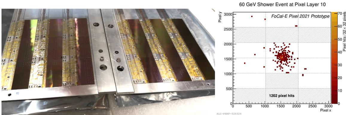
**Figure 2:** Left: Two pixel half-layers with ALPIDE chips mounted on flex PCBs. Together they form a full prototype pixel layer with 18 ALPIDE chips. Right: Display of an electron shower event at 60 GeV in FoCal-E Pixel layer 10. The shaded areas represent ALPIDEs which had to be excluded from data taking because of failures.
