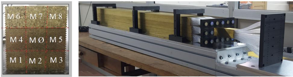
**Figure 1:** Front (**left**) and side (**right**) view of the em-size prototype before the connection to the light sensors (PMTs and SiPMs). The fibres from the external modules (M1-M8) are bundled to match the PMTs' window while the longer fibres from the central module (M0) are connected to a patch panel to be interfaced with SiPMs.
