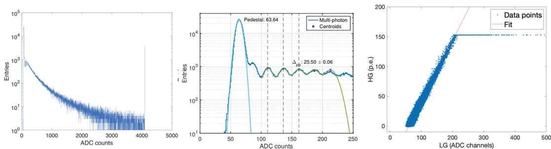
**Figure 2:** Left: HG spectrum of a SiPM for 6 GeV electrons. Centre: x-zoom of the same spectrum, showing the photoelectron peaks. Right: Correlation between the LG and the HG signals.
