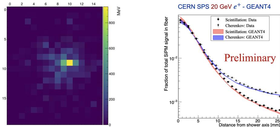
**Figure 4:** Left: Event display for the energy deposition of a 6 GeV electron in module M0. The colour in each box is proportional to the energy-calibrated signal recorded by each SiPM. Right: Lateral profile of showers produced by 20 GeV electrons in the calorimeter, separately for the scintillation and Cherenkov signals. The test beam data are compared to the results obtained with a Monte Carlo simulation that describes the CERN experimental setup.
