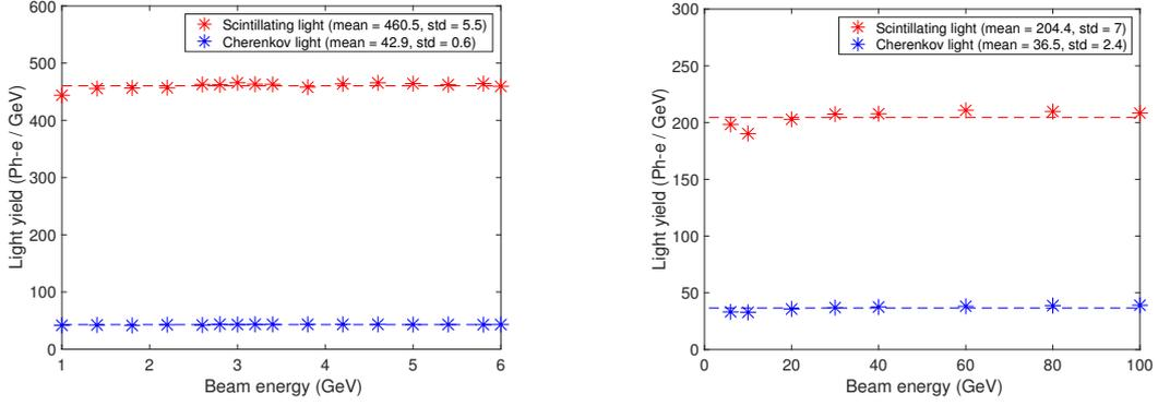
**Figure 3:** Average number of scintillation and Cherenkov photo-electrons/GeV detected by the central module as a function of the electron beam energy. Left: DESY results. Right: CERN results.
