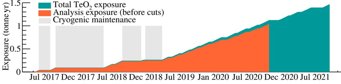
**Figure 2:** Exposure accumulated by CUORE (teal), along with the exposure used for this analysis (orange). Parts of 2017 and 2018 were dedicated to maintenance and optimization of the cryogenic set-up. Data releases on the search for  $0\nu\beta\beta$  from the CUORE Collaboration are from 2017 [2], 2019 [3] and most recently 2022 [4]. Figure from Ref. [4].
