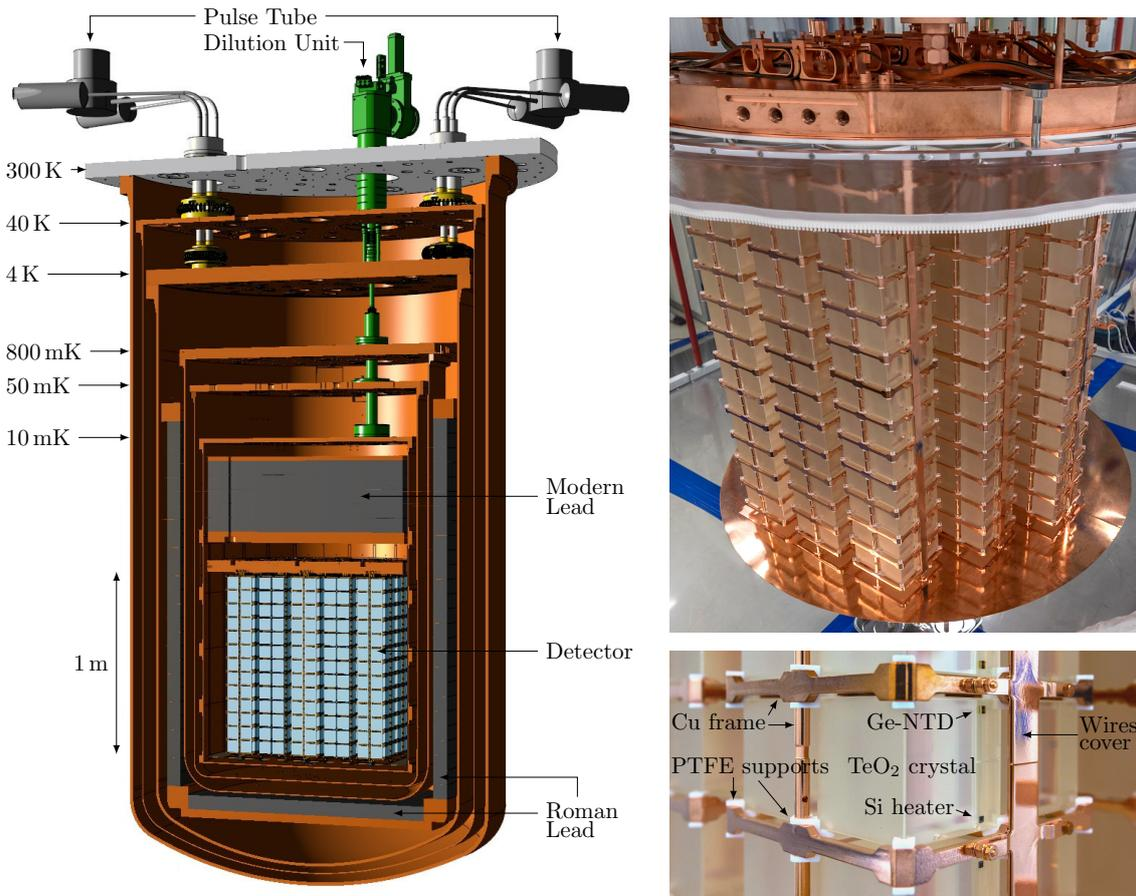
**Figure 1:** (Left) Rendering of the CUORE cryostat. The different thermal stages, vacuum chambers, cooling elements and lead shields are indicated. (Right) The detector after installation and a zoomed view on one of the calorimeters. Figure from Ref. [4].
