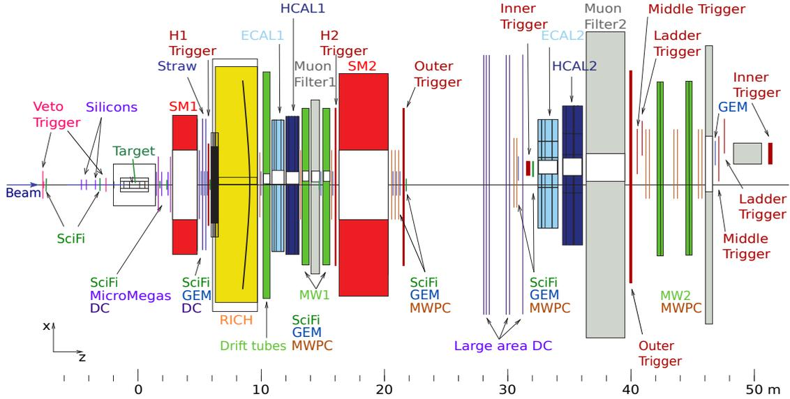
**Figure 1:** Sketch of a top view of the experimental setup of the open geometry forward spectrometer forming the basis of the AMBER setup. Shown is the COMPASS setup for the 2021 campaign. The target region will be specifically adapted for the measurements described in these proceedings. Note the excellent particle identification and muon tracking capabilities of this setup.
