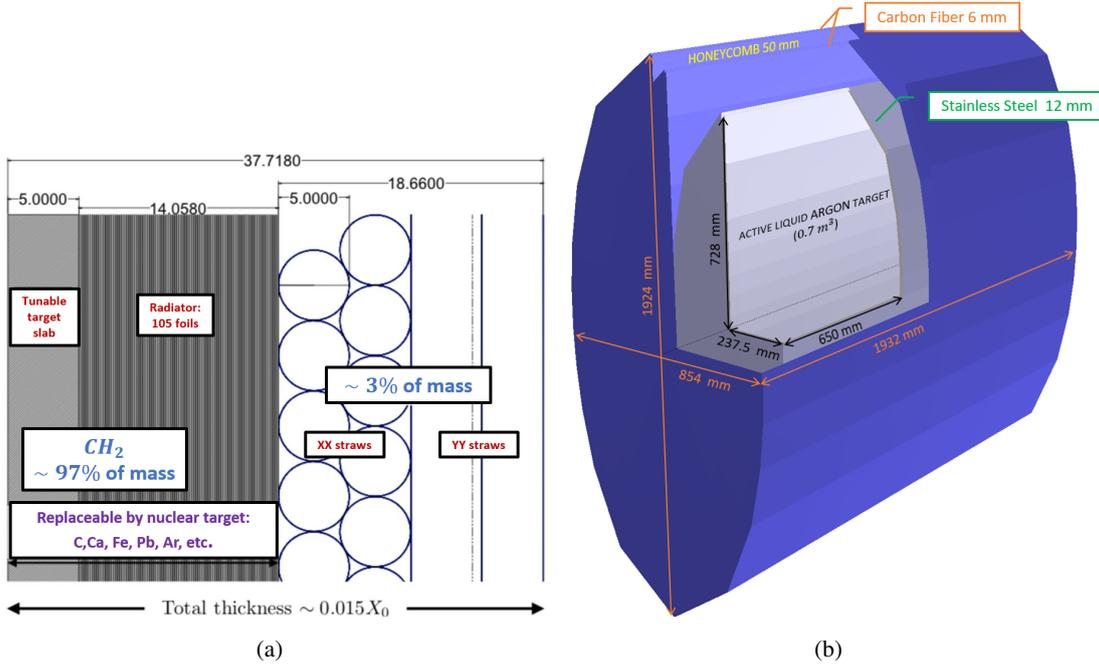
**Figure 2:** (a) Drawing of an STT module ( $xy$  section,  $z$  is the beam axis and  $x$  the B field axis) made of: (i) tunable  $\text{CH}_2$  target; (ii) radiator foils for  $e^\pm$  ID; (iii) four straw layers  $\text{XXYY}$ . (b) GRAIN cryostat simulation with: (a) inner vessel in stainless steel, (b) external vessel combination of honeycomb and carbon fiber layers.
