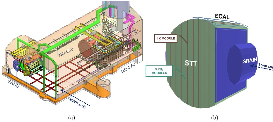
**Figure 1:** (a) DUNE ND complex components. (b) Simulation of the SAND inner volume, with an active LAr target (GRIN) upstream, followed by the tracking system (STT). The electromagnetic calorimeter (ECAL) surrounds the STT and GRIN offering a  $4\pi$  coverage.
