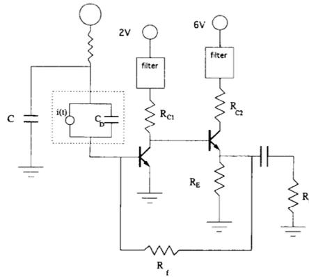
Fig.5 Front-end preamplifier of the COSIDE experiment (early 90s).
