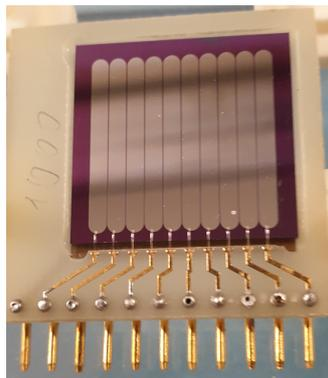
Fig.6 Silicon detector of the COSIDE experiment.
