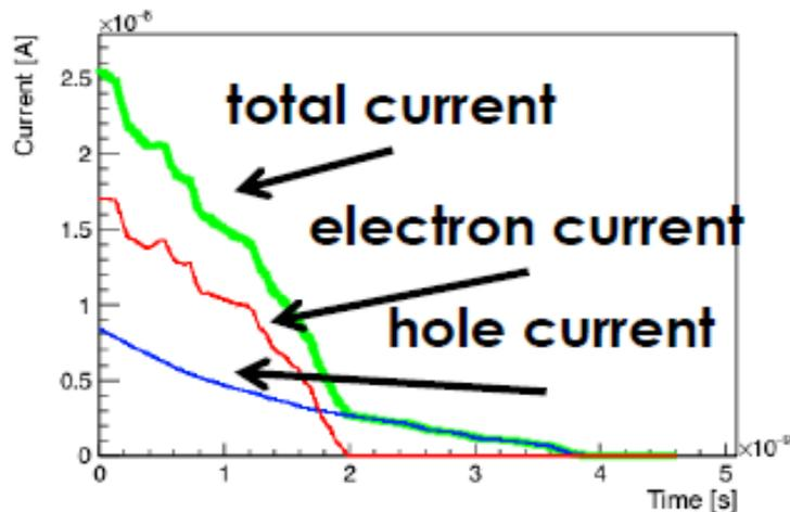
Fig.4 Current pulse in a typical planar silicon detector: Due to the different mobilities of the holes and of the electrons, the electron contribution last less (around 2 ns instead of 4 ns) and has higher current amplitude compared to the hole current. The usual approach of integrating current pulses leads (in this case) to a charge pulse having about 3 ns risetime while using current pulses the rise-time may reach ideally the value of 5 ps (not shown in the graph because too short).
