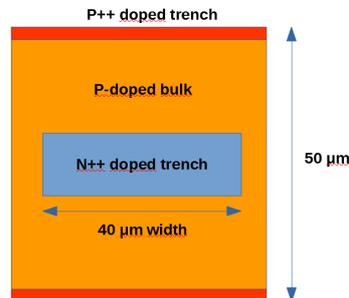
Fig.3 TIMESPOT detector layout (one cell) seen from top.
