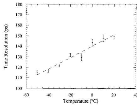
Fig. 7 Time-of-flight resolution versus temperature of the COSIDE detector.
