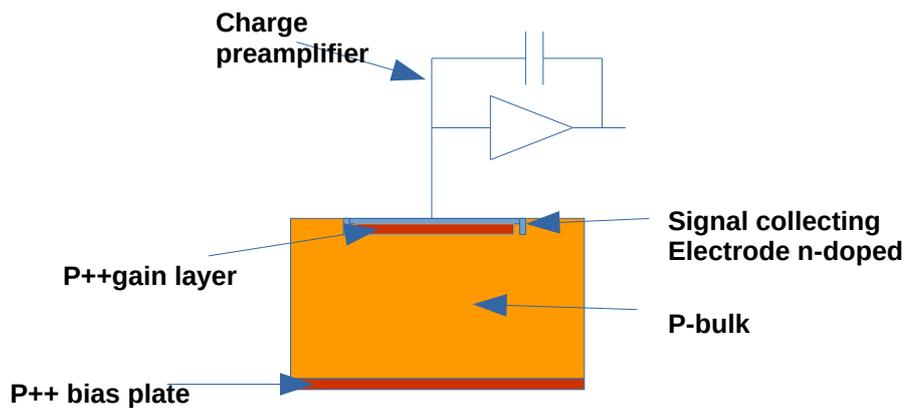
Fig.2 Low Gain Avalanche device basic scheme
