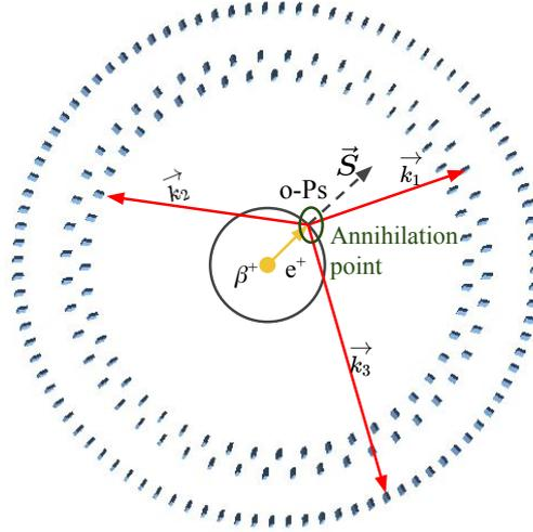
**Figure 1:** Schematic view of a 3-photon o-Ps annihilation event recorded in the prototype of 3-layer J-PET detector.  $^{22}\text{Na}$  source (yellow dot) emitting  $\beta^+$  is placed inside the vacuum-filled annihilation chamber coated with silica aerogel.
