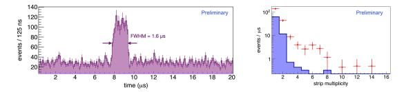
**Figure 4:** The left plot shows the event time distribution from the LAPPD. Shown is the time from the beam acquisition window start to the event timestamp. An excess of events with a FWHM of  $1.6 \,\mu$ s can be seen, which matches the BNB beam window. The right plot shows the strip multiplicity with the rate normalized to events/ $\mu$ s for on-beam data (red) and off-beam data (blue).
