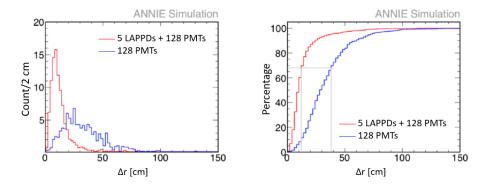
**Figure 3:** ANNIE simulation for, on the left side, the vertex and on the right side, the direction resolution for reconstructed events with only PMTs (blue) and PMTs and 5 LAPPDs (red). [3]
