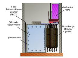
Figure 1: Schematic representation of the ANNIE detector setup. [1]
