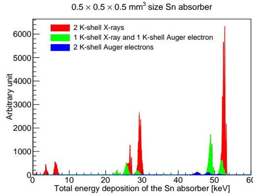
**Figure 1:** Total energy deposition of the tin absorber ( $0.5 \text{ mm}^3$  cubic, density =  $7.265 \text{ g/cm}^3$ ) for the simulated  $2\nu2\text{K}$  events (colored stacked histograms). Each color corresponds to 2 X-rays emission events (red), 1 X-ray and 1 Auger electron emission events (green), and 2 Auger electrons emission events (blue), respectively.
