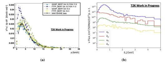
Figure 6: (a) Pion yields from G4JNUBEAM simulations (markers) and NA61/SHINE data (solid line) for the last 18 cm downstream of the target in the 20-40 mrad angular range and (b) G4JNUBEAM neutrino fluxes at ND280 (for a horn current of 320 kA).
