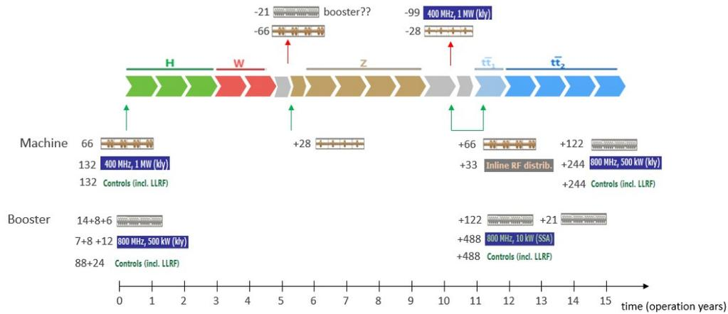
Figure 8: Alternative RF staging scenario for collider and booster ring (Courtesy O. Brunner).
