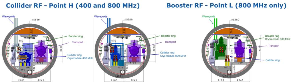
**Figure 6:** Tunnel cross sections in the FCC-ee RF straight sections. In each of the three images, the right-hand cryomodule, shown on a small vehicle, is being transported past an installed cryomodule, on the left, which is connected by waveguide to the RF power source in the klystron gallery (located above) and by cryogenic jumpers to the cryogenic distribution line, on the far left (Courtesy F. Valchкова and F. Peauger).
