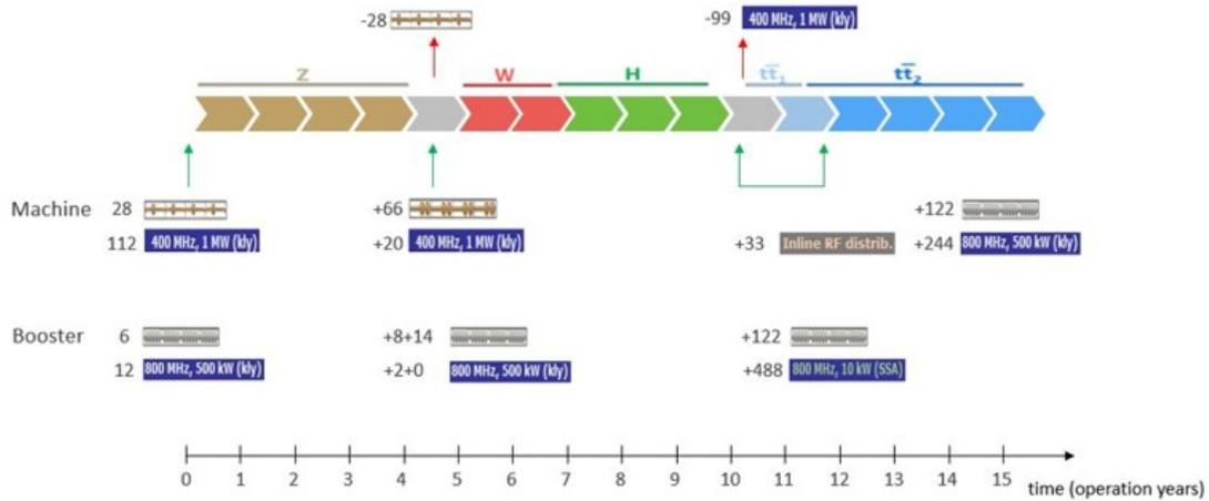
Figure 7: Baseline RF staging scenario for collider and booster ring (Courtesy O. Brunner).
