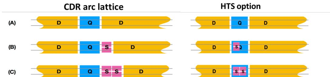
**Figure 4:** Three different types of short straight sections in the FCC-ee according to the 2018 CDR layout (left) and when using nested HTS quadrupole and sextupole coils (right) (Courtesy M. Koratzinos).
