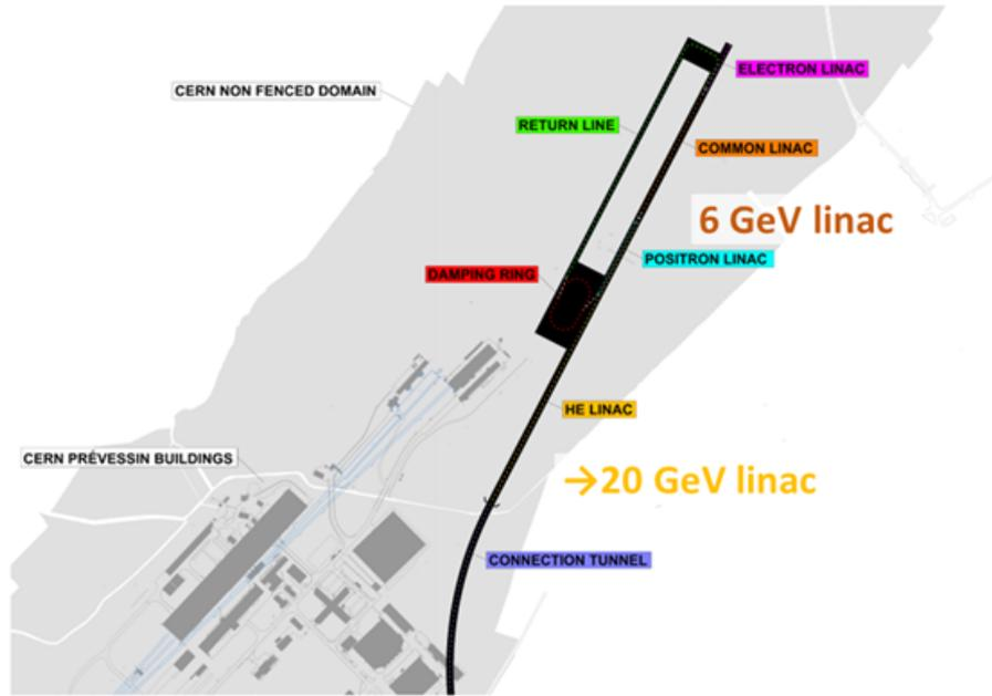
**Figure 5:** Basic and extended FCC-ee pre-injector complex located on the CERN Prévessin site (Courtesy T. Watson and W. Bartmann).
