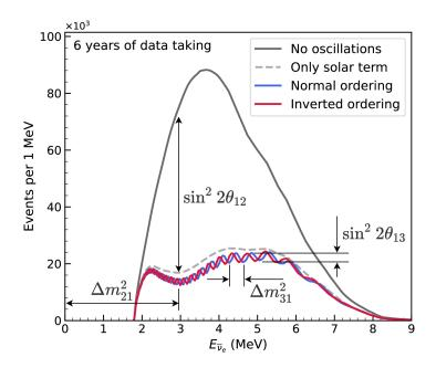
**Figure 2:** JUNO aims to measure the mass ordering using the small differences in the neutrino energy spectra assuming normal ordering (blue line) and inverted ordering (red line).
