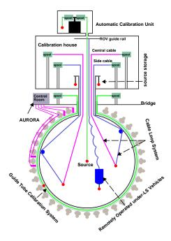
**Figure 5:** Overview of the calibration system (not to scale), which includes the Automatic Calibration Unit (ACU), Cable Loop Systems (CLS), the Guide Tube (GT), and the Remotely Operated Vehicle (ROV). The AURORA is an auxiliary laser diode system to monitor the attenuation and scattering length of the LS.
