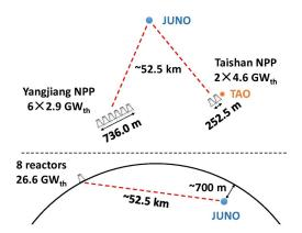
**Figure 1:** JUNO detector is located near the city of Kaiping, Guangdong province in southern China. It has a baseline of 52.5 km to the two nearest nuclear power plants, Taishan and Yangjiang. The central detector is  $\sim 700$  m under the ground level. Close to one core of the Taishan NPP will be mounted JUNO-TAO to measure the reactor neutrino spectrum [1].
