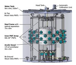
**Figure 4:** Layout of the OSIRIS detector. It is possible to divide OSIRIS into the Inner Detector (ID) which is formed by the LS volume and the inner PMT array and the Outer Detector (OD) which uses the shielding water as a Cherenkov muon veto.
