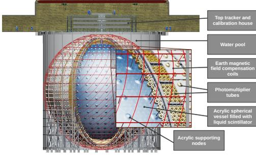
**Figure 1:** Schematic view of the JUNO central detector and other main components
