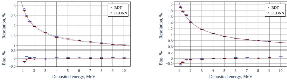
**Figure 3:** Energy reconstruction performance for BDT and FCDNN: a) JUNO detector and b) TAO detector.
