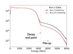
**Figure 4:** The decay positron energy spectrum using the Run-1 style clustering (blue) and the improved Run-2/3 style clustering (red). The high energy tail, which contains pileup-only events, shows that the level of pileup has been reduced by a factor of four.
