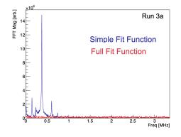
**Figure 2:** Fast Fourier transform of the Run-3a fit residuals using a simple fit model in blue (muon decay and g - 2 oscillation only) and the full model in red (see text). The peaks in the simple fit — due to unaccounted for beam frequencies — are removed in the full fit.
