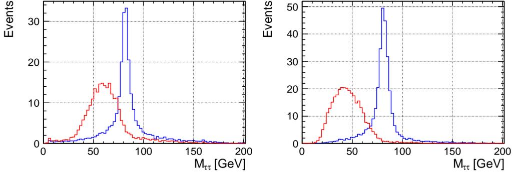
**Figure 2:** Reconstructed invariant mass of the two tau candidates, before (red) and after (blue) the collinear energy correction. Distributions are shown for signal of light scalar production with mass of 80 GeV, for hadronic (left) and semi-leptonic (right) event selection.
