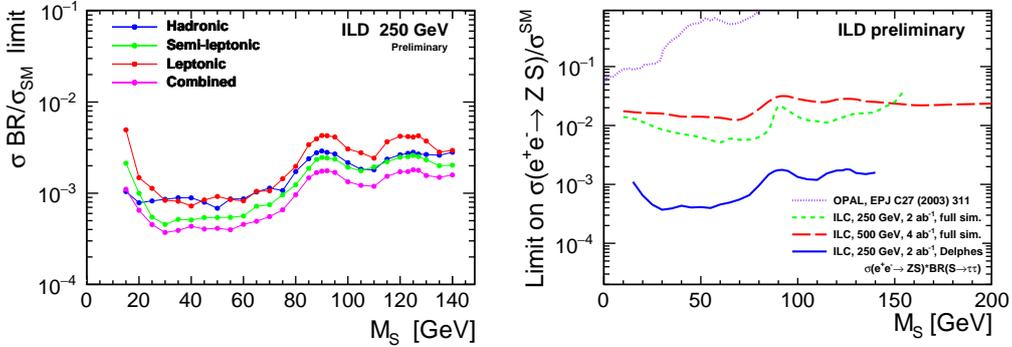
**Figure 5:** Cross section limits in di-tau channel expected for ILC running at 250 GeV, resulting from the selection based on the BDT response cut, as a function of the assumed scalar mass. Limits expected from the combined analysis of all data are compared with limit estimates for different signal channels (left) and with limits resulting from earlier, decay channel independent studies (right).
