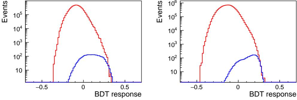
**Figure 4:** Example of the BDT response distribution for signal (blue) and background (red) events, for new scalar mass of 80 GeV. The signal cross section is set to 1% of the SM Higgs boson production cross section at given scalar mass. The BDT classification was applied to the combined data set, including all beam polarisation combinations, for the loose event selection.
