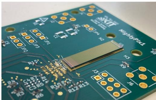
**Figure 2:** MightyPix1 wire-bonded to a PCB for testing. (Photograph courtesy of Karlsruhe Institute of Technology.)
