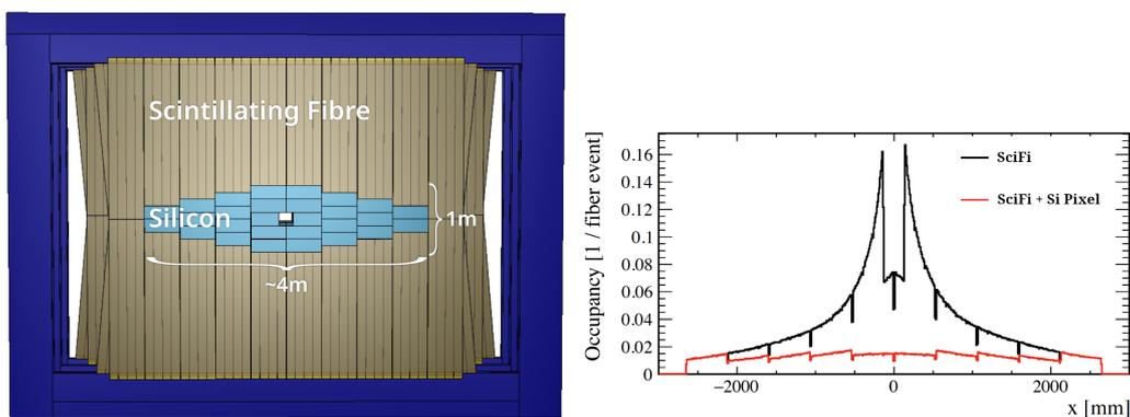
**Figure 1:** L: Mighty Tracker: the outer region shows the scintillating fibre tracker, and the inner region (blue) shows the silicon pixel layer. R: The occupancy of the scintillating fibres without and with the silicon layer.
