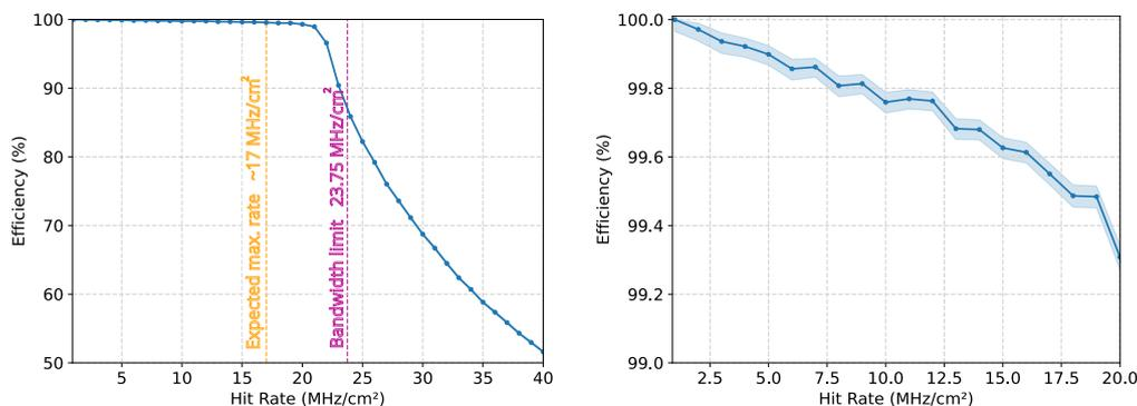
**Figure 5:** L: Simulated MightyPix1 readout efficiency vs. hit rate The expected maximum rate of  $17 \text{ MHz/cm}^2$  and maximum available bandwidth of  $20 \text{ MHz/cm}^2$  are indicated by vertical lines R: A zoomed view showing the small efficiency loss above 99%.
