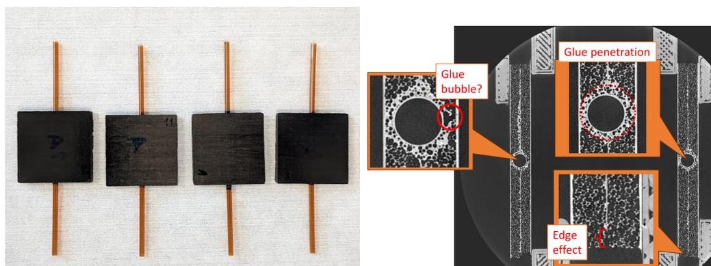
**Figure 4:** L: Prototype carbon-foam substrates R: X-ray tomography of substrate samples ((pictures courtesy of U. Manchester).
