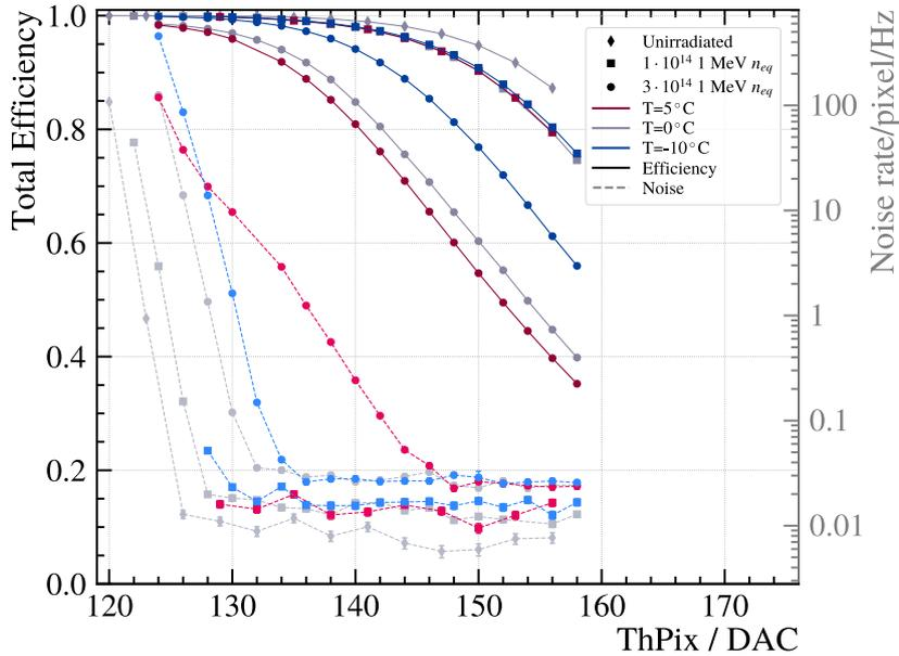
**Figure 6:** ATLASPix 3.1 efficiency and noise as a function of pixel hit threshold (in DACs). Details are described in the text.
