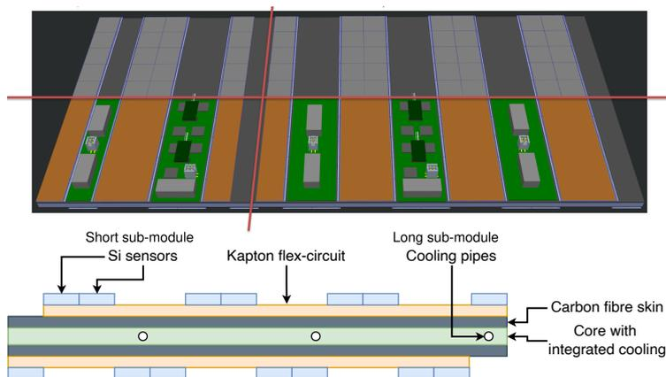
**Figure 3:** T: Current design of the inner short modules. The modules are sub-divided into sub-modules. B: Module cross-section.
