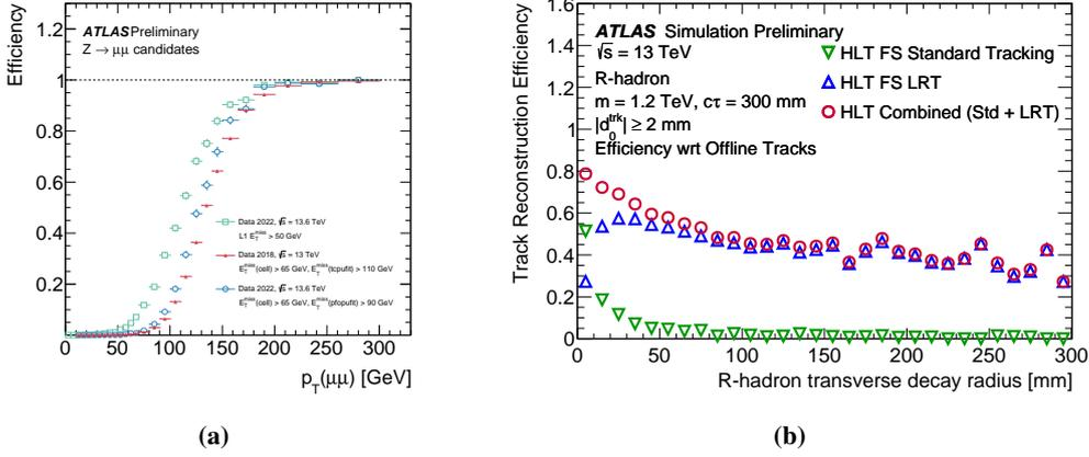
**Figure 2:** Left: Efficiencies for the missing energy trigger measured with  $Z \rightarrow \mu\mu$  events where  $p_T(\mu\mu)$  is used as a proxy for  $E_T^{\text{miss}}$  in 2018 and 2022 data. Ref: [9]; Right: Track reconstruction efficiency for the decay products of a 1.2 TeV supersymmetric R-hadron as a function of the truth transverse decay radius of the R-hadron for two different HLT tracking strategies and their combination. Ref: [10]
