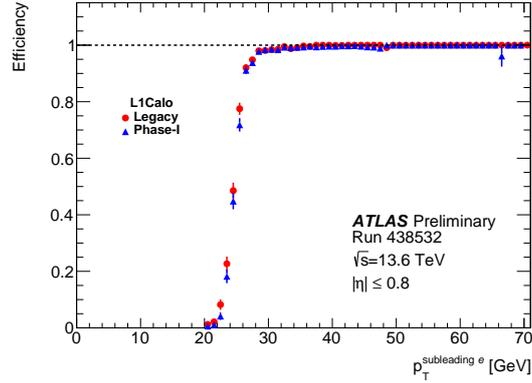
**Figure 1:** L1Calo single electron trigger efficiencies in the inner calorimeter barrel  $|\eta| < 0.8$ , measured using  $Z \rightarrow ee$  events with the tag-and-probe method, as a function of subleading electron  $p_T$ , for the Run 2 system (red) and for the Run 3 (eFEX-based) system (blue). Source: [2]
