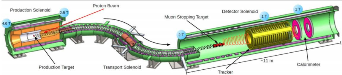
**Figure 1:** Schematic view of the Mu2e apparatus
