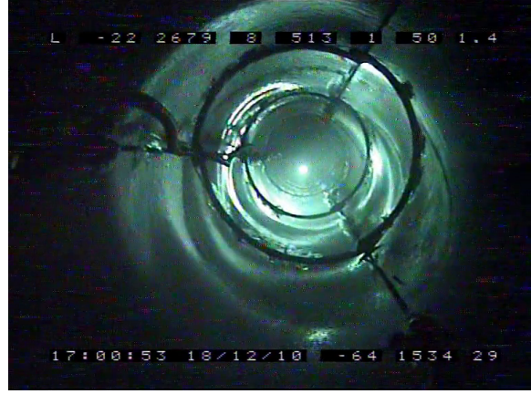
Figure 3: Video still frame of the lower camera looking up the drill hole towards the upper camera which is emitting light.
