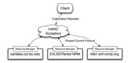
Figure 1: The HARC architecture, showing the relationship between the client, the Acceptors, and the Resource Managers (RMs).
