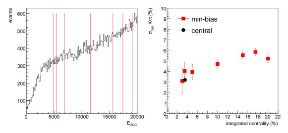
**Figure 3:** Left picture: distribution of the energy deposited in the Zero Degree Calorimeter (ZDC) of NA49 in Pb + Pb collisions at 158A GeV beam energy. Vertical lines show cuts, which correspond to 3%, 3.5%, 5%, 10%, 15%, 17.5% and 20% centrality bin size. Right picture: dynamical fluctuations of the  $K/\pi$  ratio as a function of the centrality bin size in Pb + Pb collisions at 158A GeV beam energy.
