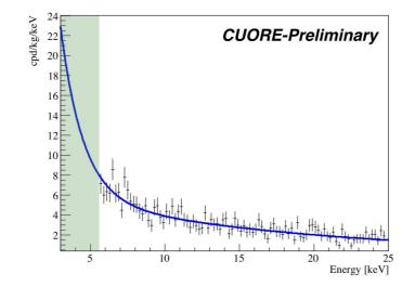
**Figure 6:** Differential rate at low energies obtained combining data from the three bolometers having the energy threshold at 3 keV. The region below 5 keV is not shown, since it is still under study (see text). The data are fitted with a double exponential decay, and the fit function is used as model of the CUORE background.
