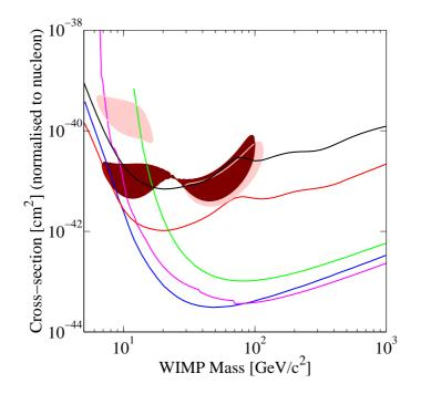
**Figure 7:** CUORE(5y) (in red) and CUORE-0(3y) (in black) expected sensitivities compared to the actual limits on WIMP-nucleon elastic scattering cross section. DAMA/LIBRA  $3\sigma$  evidence with ion channeling in dark red and without ion channeling in pink, Edelweiss II in green, XENON100 in blue, CDMS in magenta.
