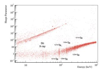
**Figure 5:** Shape parameter distribution of all the events in the range 5-1000 keV for one of the three bolometers used in the data analysis. The band at low values of the shape parameter is populated by signal events, where the lines generated by metastable Tellurium isotopes are visible. At higher values there are triggered mechanical vibrations and spikes.
