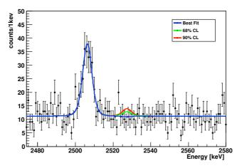
**Figure 1:** CUORICINO energy spectrum in the region of interest. The line at 2505 keV is due to  $^{60}$ Co contamination of the materials surrounding the bolometers. No peak is found at the expected 0*v*DBD energy of 2527 keV.
