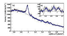
**Figure 1:** The  $K_S K^{\pm} \pi^{\mp}$  (a) and  $K^+ K^- \pi^+ \pi^- \pi^0$  (c) mass spectra. The solid line is the fit result. The dashed line represents non-resonant background. The plots (b) and (d) show background subtracted spectra for the mass range 3.3–3.7 GeV/ $c^2$ .
