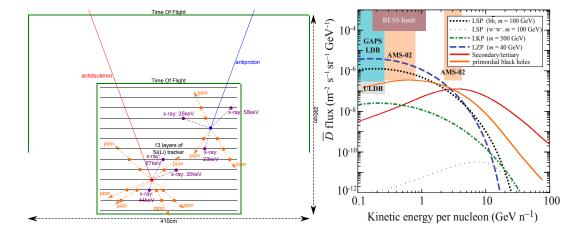
Figure 2: *Left*) GAPS detector concept with antiproton and antideuteron signatures. *Right*) Antideuteron sensitivity for GAPS and AMS-02 (superconducting magnet setup) with fluxes from different models [11].
