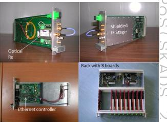
Fig. 8: Different views of the IF board and 8 boards already assembled in a 19" rack.
