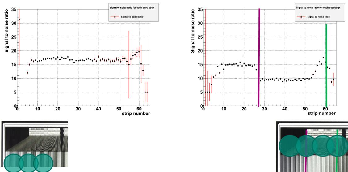
**Figure 13:** Signal-to-noise ratio of a structure with integrated pitch adapter. On the left plot the source is above the normal region, on the right plot the source is above the pitch adapter region[4].
