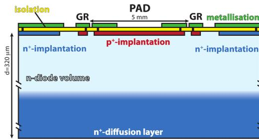
**Figure 3:** Cut through a diode on deep diffused floatzone-silicon [3].
