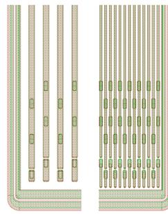
**Figure 6:** Multi geometry strip sensor for optimizing layout parameters.
