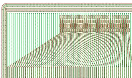
**Figure 7:** Baby sensor with metal routing integrated in first metal layer.
