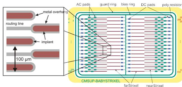
**Figure 8:** Short strip sensor with routing of the inner strips in the first metal layer.
