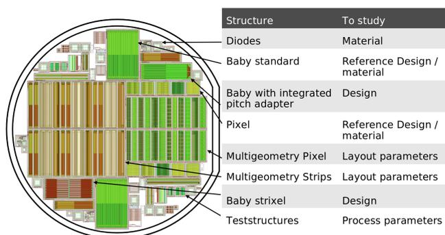
**Figure 2:** Wafer of the campaign with the different structures.
