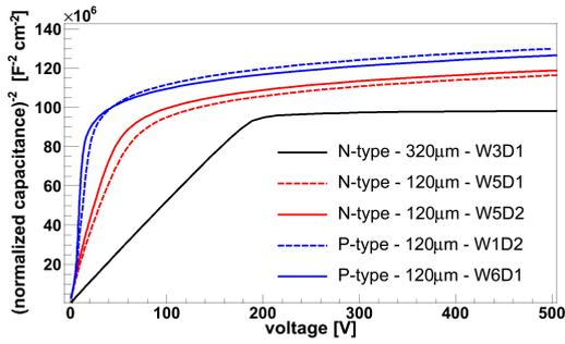
**Figure 10:** Capacitance voltage characteristics of different deep diffused materials.
