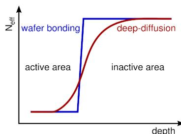
**Figure 9:** Interface shape of deep diffusion vs wafer bonding.
