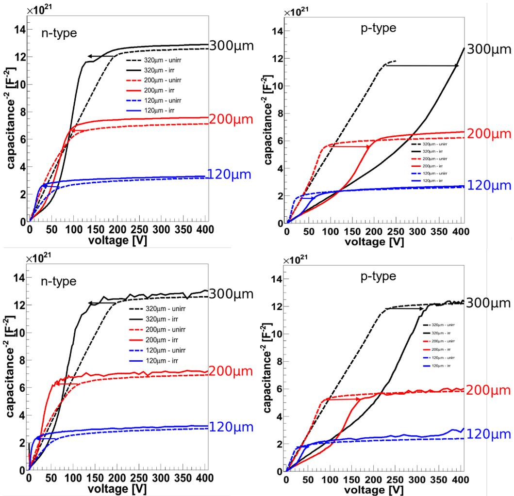
**Figure 12:** Capacitance voltage characteristics for different thicknesses and materials, before and after irradiation with neutrons (upper plots) and protons (lower plots).
