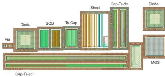
**Figure 4:** Teststructure with the different sub-structures for process qualification.
