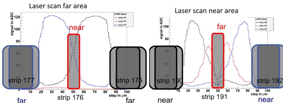
**Figure 14:** Signal of a short strip structure. On the right the laser scan was performed in the near area, on the left it was performed in the far area. The boxes symbolise the strips whose signal is shown. The outer strips are the ones, that should show the signal, the middle one should not [4].
