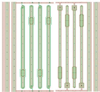
**Figure 5:** Multi geometry pixel sensor for optimizing layout parameters.
