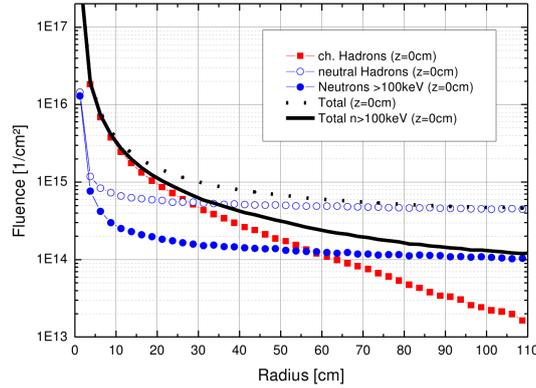
**Figure 1:** The black line shows the total fluences for different radii in the central region for an integrated luminosity of  $3000 \text{fb}^{-1}$  [1].
