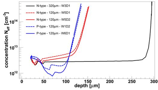
**Figure 11:** Profile of effective charge carrier concentration, calculated from fig. 10.
