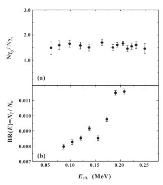
**Figure 2:** (a) Relative ratio of yields of the ground-state and first-excited captures in the  ${}^{6}\text{Li}(p,\gamma)^{7}\text{Be}$  reaction, and (b) branching ratio BR(*E*) of the  $\gamma$ -ray-to- $\alpha$ -particle from reactions of  ${}^{6}\text{Li}(p,\gamma)^{7}\text{Be}$  and  ${}^{6}\text{Li}(p,\alpha)^{3}\text{He}$ . Where all errors are of statistical origin, and *x*-axis indicates the effective energies [7].
