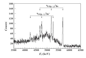
**Figure 1:** Sample  $\gamma$ -ray spectrum from the p+<sup>6</sup>Li radiative capture reaction obtained at energy of *E*=94 keV.
