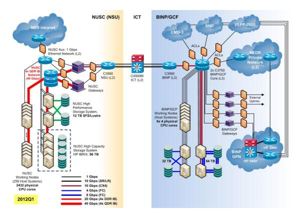
Figure 2: Network, computing and storage resources integration layout for NUSC and BINP/GCF computing facilities by means of NSC/SCN supercomputer network.
