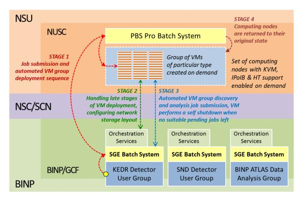
Figure 3: Batch system integration layout between the detector experiment user groups on the BINP side and NUSC computing facility. Four stages of a specific virtual machine group deployment on the NUSC side are shown.
