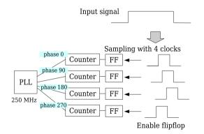
Figure 6: The schematic of MHTDC in FPGA.
