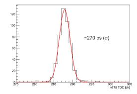
**Figure 5:** The distribution of TDC obtained by injecting a charge.
