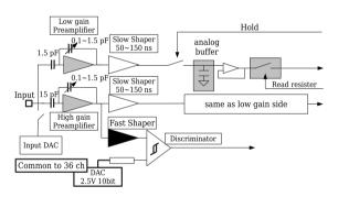
**Figure 2:** The Schematic of one channel in EASIROC.
