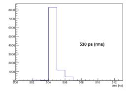
**Figure 7:** The distribution of MHTDC obtained by injecting a charge.
