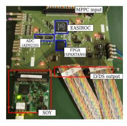
Figure 3: Picture of the evaluation board.
