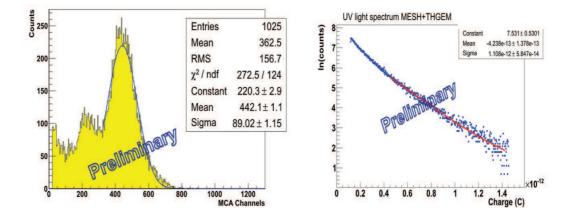
**Figure 3:** Amplitude spectra obtained with the hybrid detector prototype. Left: using the  ${}^{55}Fe$  source; estimated gain:  $2.5 \cdot 10^5$ . Right: illuminating in single photon detection mode; estimated gain:  $\approx 1.2 \cdot 10^6$
