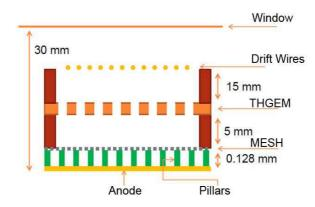
**Figure 2:** Scheme of a hybrid detector (not to scale). The geometrical parameters refer to the detector used to obtain the results presented in sec. 3
