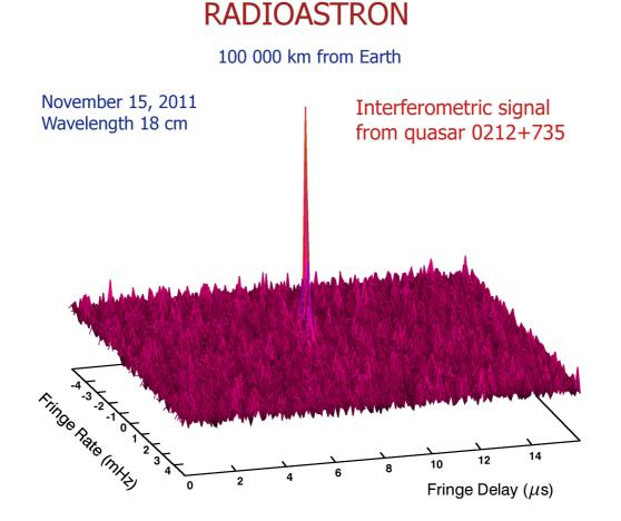
**Figure 2:** The first fringes found by the Space-VLB interferometer RadioAstron. Interference signal from the quasar 0212+735 on a 8,100 km projected baseline between RadioAstron and the 100-m MPIfR radio telescope near Effelsberg, Germany, observed on November 15, 2012. The wavelength of the observations was 18 cm. The plot shows the fringe amplitude versus residual delay and residual fringe rate in a single 16 MHz wide channel.
