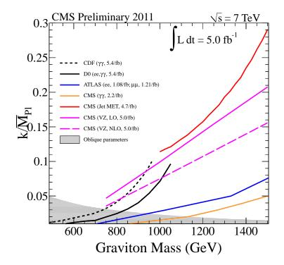
**Figure 3:** Observed and expected 95% CL exclusion limits for a counting experiment and comparison with the theoretical predictions in RS Graviton models for the combination of electron and muon channels. The limits are calculated with the frequentist CLs statistical method. The resonance of the hypothetical particle is considered narrow with respect to the experimental resolution.
