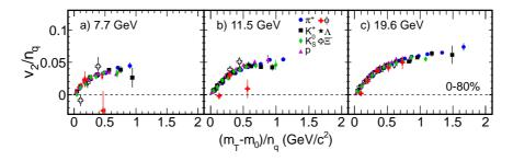
**Figure 2:** (Color online) The elliptic flow scaled by number-of-constituent quark  $(n_q)$  as a function of  $(m_T - m_0)/n_q$  for selected particles in the Au+Au collision at  $\sqrt{s_{NN}} = 7.7$ , 11.5 and 19.6 GeV for 0-80% centrality [12, 13]. Error bars are only statistical uncertainties.
