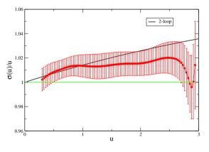
**Figure 5:** The growth rate  $\sigma(u)/u$  as a function of *u* with statistical error. Two-loop perturbative value (black line) is also plotted for comparison. The horizontal (green) line denotes unity line, where the beta function is consistent with zero.
