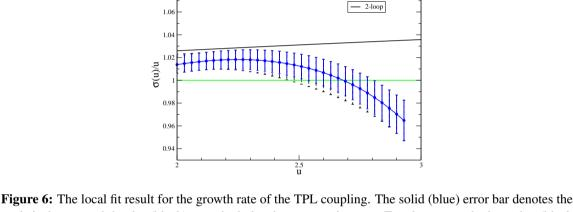
Figure 6: The local fit result for the growth rate of the TPL coupling. The solid (blue) error bar denotes the statistical error and the dot (black) error includes the systematic error. Two-loop perturbative value (black line) is also plotted for comparison. The horizontal (green) line denotes unity line, where the beta function is consistent with zero.
