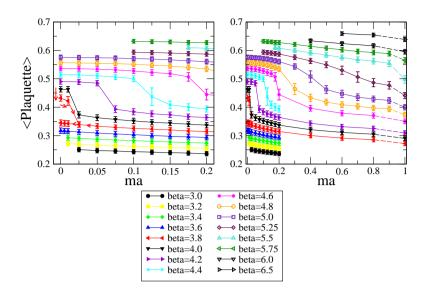
**Figure 2:** Plaquette values for several  $\beta$  and *ma* on  $(L/a)^4 = 4^4$  lattice. The data at *ma* = 1 on the right panel denotes the quenched QCD. The small (red) arrows near the massless at  $\beta = 3.8$  on the left panel shows the detailed history of the thermalization. The other data are thermalized from massive to massless direction.
