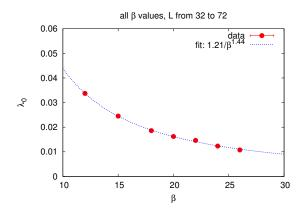
**Figure 1:**  $\lambda_0$  vs.  $\beta$  from simulations of SU(2) lattice gauge theory in (2+1) dimensions at various couplings and lattice volumes. The best fit to data is  $\lambda_0 \propto \beta^{-1.4}$ , which differs from the expected  $\beta^{-2}$  dependence and indicates that  $\lambda_0$  diverges in the continuum limit.
