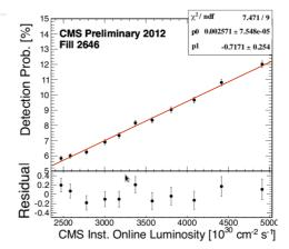
Figure 1: Calibration scan results comparing BCM1F to other luminosity subsystems.
