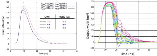
Figure 3: Amplifier response to MIP signals showing fast rise time for various bias settings.
