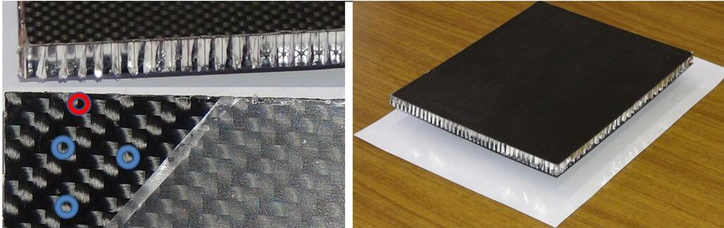
**Figure 5:** Samples of carbon plastic mirror. Left: flat sample, on top - three layer construction, on bottom - edge of the sample with 4 “points” for roughness estimations (reflective surface partially covered by protective film). Right: spherical sample with sizes  $18 \times 20 \text{ cm}^2$  and radius of curvature 741 cm.
