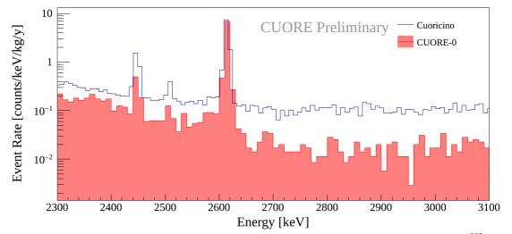
*Figure 3: Zoom of the spectra shown in Figure 2 in the energy region across the* <sup>208</sup>*Tl peak.*
