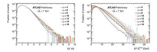
**Figure 1:** Right: the distribution of Event Filter (EF)  $E_{\rm T}^{\rm miss}$  for different values of pile-up collisions  $\mu$ . Left: the distribution of EF XS for different values of  $\mu$ . The comparison shows that the pile-up dependence is much reduced by using EF XS instead of EF  $E_{\rm T}^{\rm miss}$ . [5]
