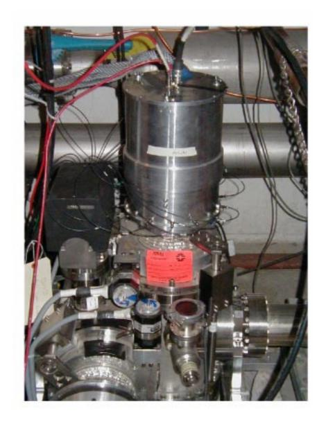
**Figure 2:** Picture of a quadrupole spectrometer installed inside the Tevatron. The TOP detector is fully equipped.
