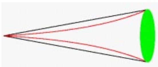
Figure 4: A cartoon to demonstrate the geometrical effect which causes structures of a given size at the epoch of recombination to appear smaller in open universes than in flat ones.
