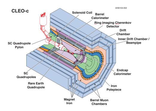
**Figure 1:** The CLEO-c detector at the Cornell Electron Storage Ring This is the latest incarnation of a detector with a more than two decade history of heavy quark physics in  $e^+e^-$  annihilation reactions.
