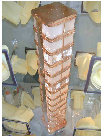
Figure 1: The CUORICINO tower inside a nitrogen-fluxed glove-box, during the final assembly of the detector.
