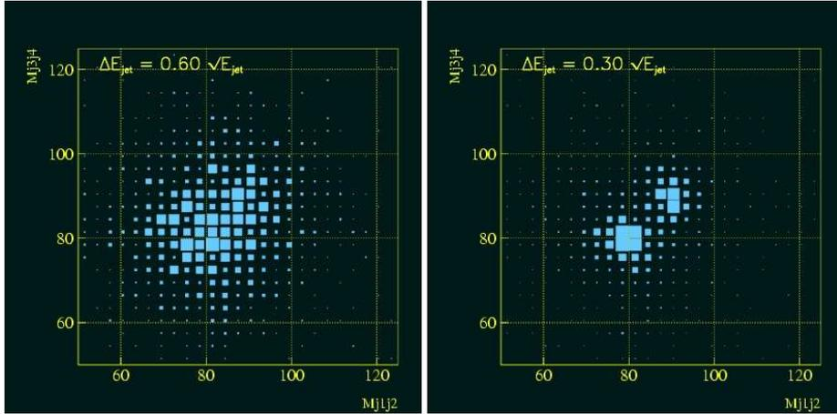
**Figure 10:** Reconstructed masses of hadronically decaying W- and Z-boson pairs in the process  $e^+e^- \rightarrow \nu\bar{\nu}WW/ZZ$  for a jet energy resolution of 60% (left) and 30% (right).
