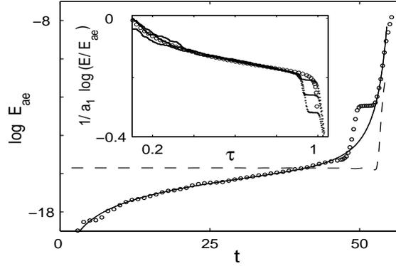
**Figure 5:**  $\log E_{ae}$  as a function of time  $t$  ( $\circ$ ) along with a fit (solid line) for the coulomb friction. Dashed line indicates the mean kinetic energy. The inset shows the collapsed curve for three different events along with a fit ( $\circ$ ).
