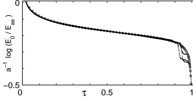
**Figure 4:** Collapsed data using  $a_1^{-1} \log(E(0)/E(\tau))$  versus  $\tau$  for three different events along with the fit shown by  $(\circ)$  for friction law with creep.
