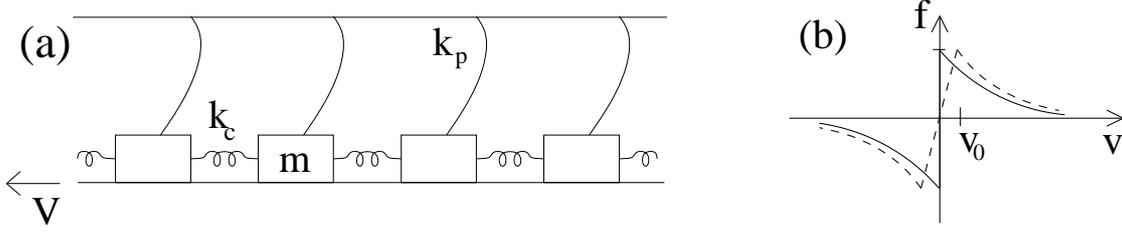
**Figure 1:** (a) The Burridge-Knopoff spring block model. (b) Friction laws: The coulomb friction law at zero velocity beyond which a smooth velocity weakening friction law (solid line). Dashed curve describes a creep branch with a similar velocity-weakening behavior.
