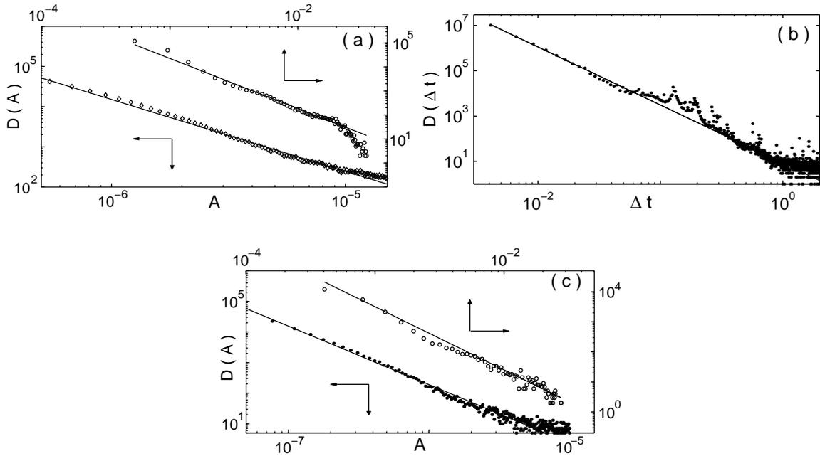
**Figure 6:** (a) Distribution of amplitude of  $R(A)$ ,  $D(A)$  versus  $A$ . ( $\diamond$ ) indicates small amplitudes and ( $\circ$ ) shows large amplitudes for  $\nu = 0.01$ , (b) Distribution of time intervals of AE events and (c)  $D(A)$  versus  $A$  for  $\nu = 0.001$ , ( $\bullet$ ) corresponds to the small amplitudes and ( $\circ$ ) that for large.
