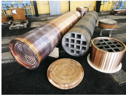
Figure 1: Canisters for spent BWR nuclear fuel. The canister consists of a cylindrical copper shell with a pressure-bearing insert of nodular iron. The outer diameter is 1.05 m and the length 4.83 m [1].
