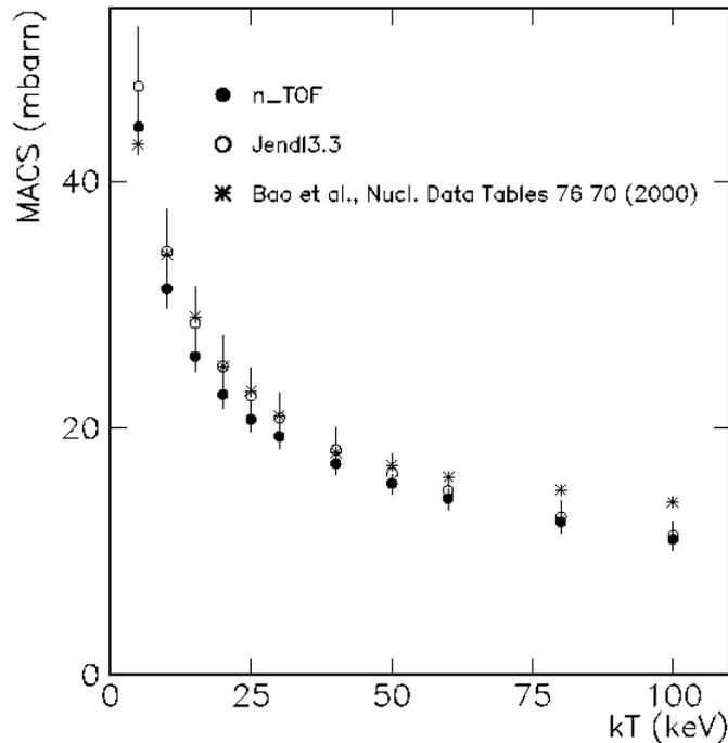
Figure 1: Comparison of MACS calculated from our  $^{90}\text{Zr}$  data (full circles), with values obtained from JENDL3.3 (open circles) and the compilation of Ref.[2] (asterisks).
