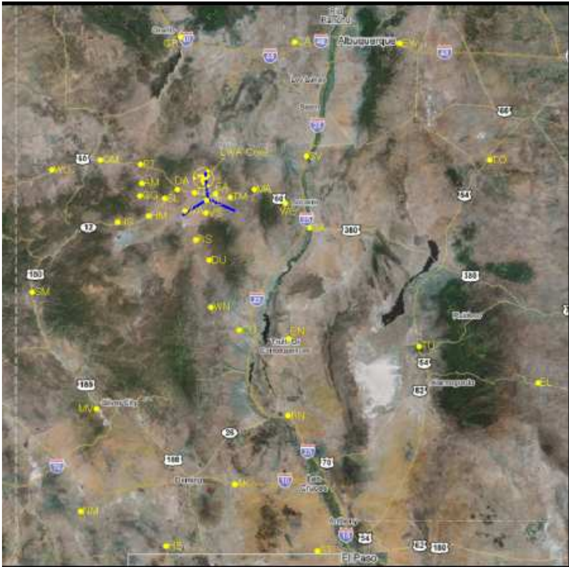
Figure 2: An illustration of how the LWA stations may be deployed across the state of New Mexico. Possible station locations are indicated as yellow dots, and the blue Y indicates the location of the VLA. Major highways and cities are also indicated, and the dotted lines indicate the state boundaries. While assessment of sites continues, this figure illustrates how 400-km baselines, producing arcsecond angular resolution, could be obtained.
