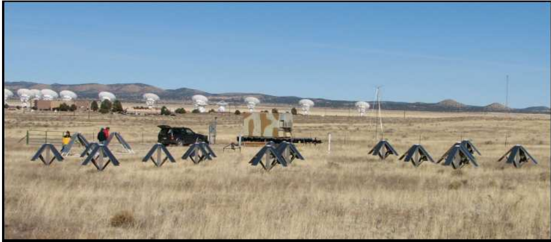
Figure 3: The Long Wavelength Demonstrator Array. The dipoles are in the foreground and are approximately 1 m high. The LWDA electronics are housed in the shed in the background. The VLA antennas are in the distance.
