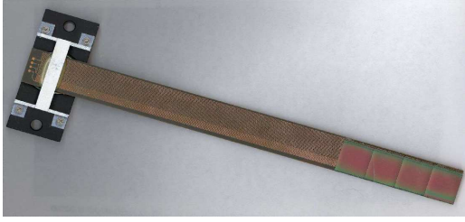
Figure 11: View of the STAR HFT ladder prototype (left) and associated material budget (right) [41]. The ladder prototype is 20 cm long and 2 cm wide, and is supported only at one end, consistently with the side-mount foreseen in the STAR HFT upgrade.
